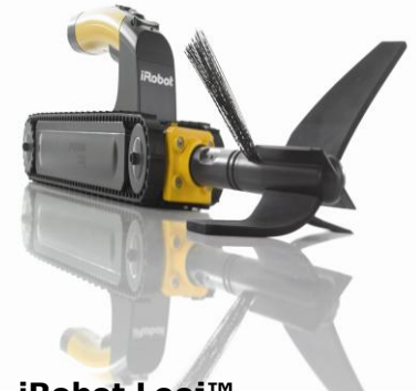
iRobot Looj™ Gutter Cleaning Robot
